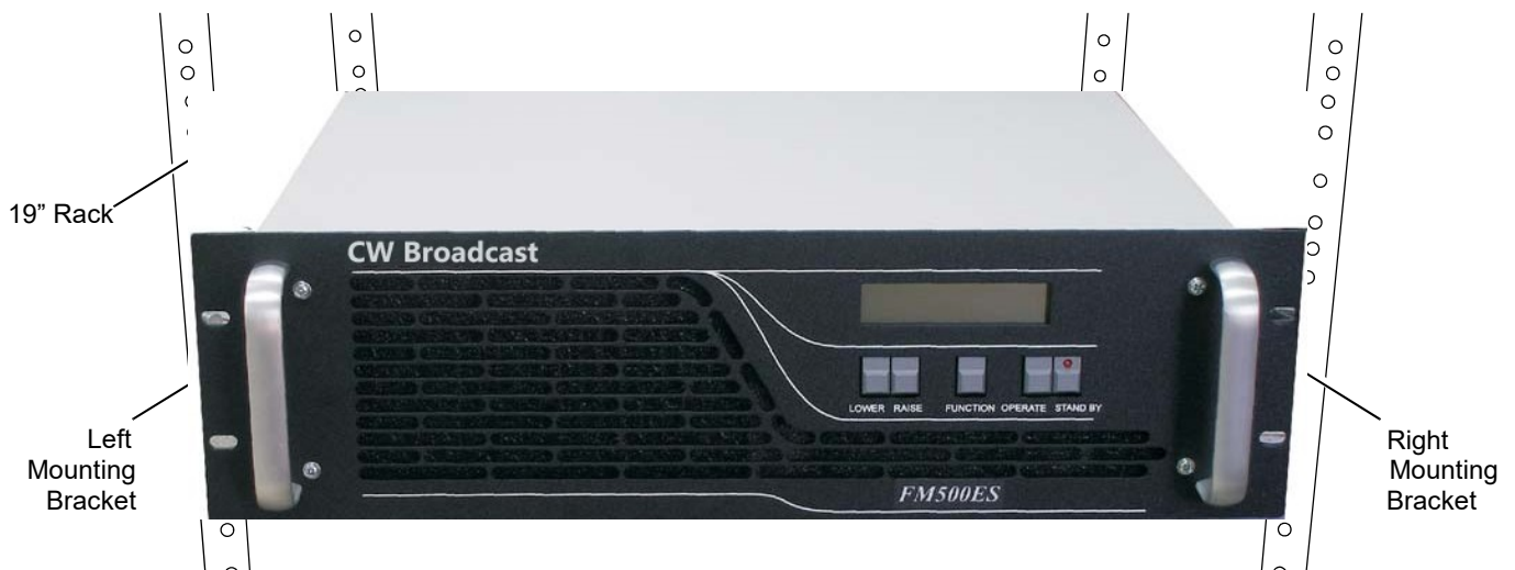
Figure 2-8. Left and Right Rack-Mount Brackets
