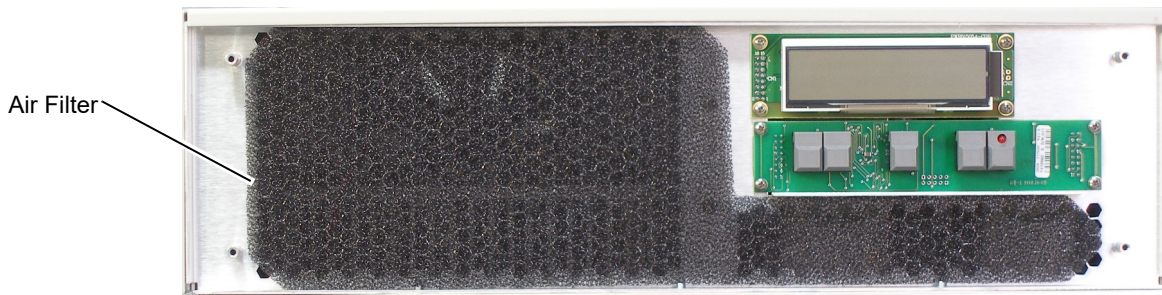
Figure 2-6. Remove the Exposed Air Filter
