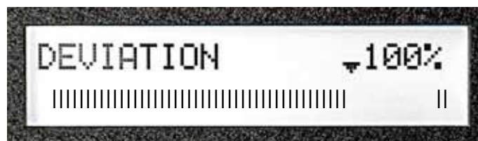
Figure 3-13. Press the FUNCTION Key to read Deviation
