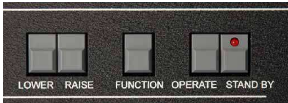
A Before power is applied to the system, the STANDBY key LED is off
