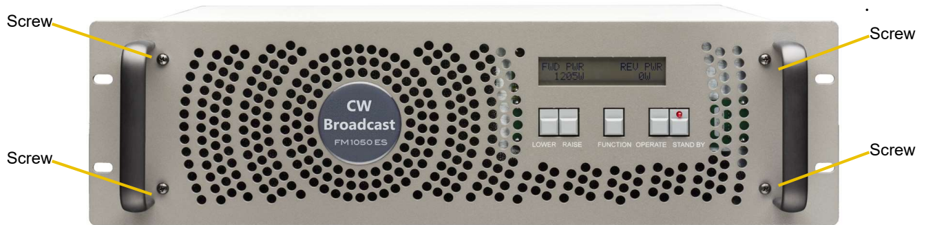
Figure 2-5. Remove the Front Panel Screws to Access the Air Filter
