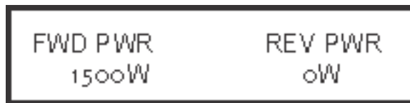
Figure 3-4a: Press the FUNCTION key to read Powers
