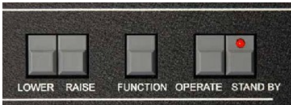
B After power is applied to the system, the standby LED is ON
