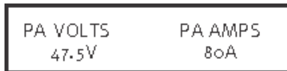
Figure 3-4b: Press the FUNCTION key to read Voltage and Current
