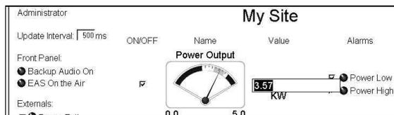
6. Note that if you set the meter pointer to extend beyond the upper scale, the meter will read overload, even if there is still range in the A/D. If autorange was previously selected in the telemetry setup, the full scale value will self-adjust.
