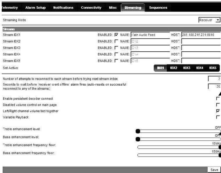
**Persistent decoder connect and retry attempts:** When persistent decoding is enabled, the SiteSentry will try each index the user defined number of retries before moving on to the next. When the last index is reached, the loop will start over until a connection is achieved.
