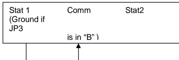
**Note:** The status “common” is a ground when JP3 is set to the “B” position (default). If JP3 is set to “A”, then comm is floating and can be used to source a voltage to the optoisolators. If sourcing a voltage, JP4 (the internal pull-up) should also be removed.
