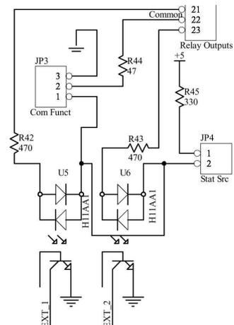
**HINT:** In default setup, turn on status inputs by connecting the trigger input to comm
