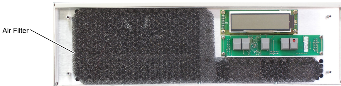
Figure 2-6. Remove the Exposed Air Filter
